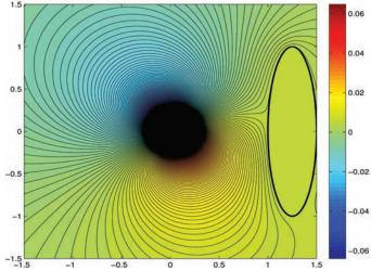
Perturbations in potential of weak electric field of fish (*Right*) caused by object (*Center*).
